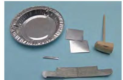
ash tray, flattened out with a rounded piece of wood, cut to size with scissors and formed around the wing leading edge.
