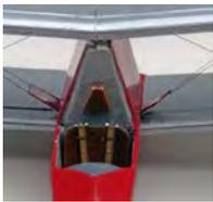
wires are the same, double, but the turn buckles at the lower wing have a protection against water. This last ones I have modelled from small pieces of disposable ashtray aluminium. The first attempt to apply the lift wires failed, because they ended up in the same hole, what I only noticed after gluing them. But that was easily corrected by drilling the holes again. The wire drops out from itself then.
