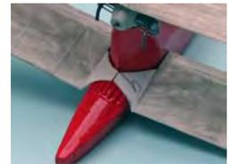
I have filled the cavities at the underside of the fairing with white glue, and have painted it white.
