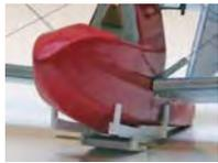
The wheels I have made from 1 mm sheet, shaped in the drilling machine with abrasive paper. The rather large holes for the axle in it, required to attach it to the drill tooling, I have made to size with pieces of the plastic tube. I have completed the structure by fitting trial and error the
