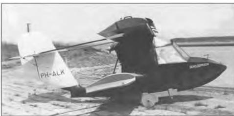
The Scheldemeeuw was also equipped with Handley Page slats on the outer parts of the upper wing, which extend automatically at low speed. I have produced these the same way as those for the Scheldemusich from the bottom of an aluminium expendable
