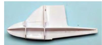
I have drilled quite a number of 1.2 mm holes in the vertical and horizontal parts where the cockpit must come. This way it will be easier to remove the excess styrene after mounting the outside fuselage panels, which are needed to give the necessary stiffness to the hull.
