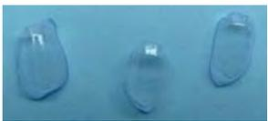
I have produced four copies of the top part by pulling heated transparent plastic over the mould. One copy was nicely brown (too hot), one was asymmetrical (the left one on the picture) and the two other had the correct shape. One jumped away in the process of cleaning, and I could not find the tiny thing anymore. The other one I adjusted trial and error to the required dimensions. A dry fit showed only gaps of some 0.1 or 0.2 mm, which can be closed with white glue after mounting.
