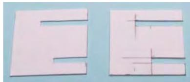
To mount the lower wings I have made two jig parts from 0.5 mm sheet, which had the correct stagger and distance between the wings, taken from the Scheldemusich drawing and the measured wing thickness. These have been
