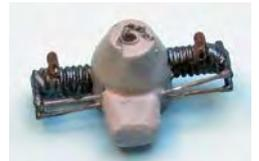
The propeller of the Scheldemeeuw is the same as that of the Scheldemusich, so I have used the drawing of that model. I have glued a copy of the drawing on a piece of 1.5 mm thick styrene, have cut out the outline and have sanded the profile in it. The spinner has been sanded from a piece of sprue. A piece of 0.5 mm brass rod finished the job.
