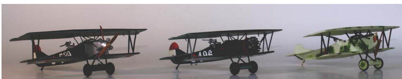
Three versions of the Fokker C.I. From right to left the original C.I with BMW IIIa engine, the upgraded C.Ia with Armstrong Siddeley Lynx engine and the (single) upgraded C.Ia with Armstrong Siddeley Mongoose engine iii .
