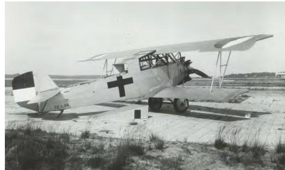
The first flight took place in February 1932. The longitudinal stability and controllability appeared to be insufficient, hence small fin was placed. Later the rudder and fin were again replaced by a larger, better shaped vertical tail plane. Also the original wheels were replaced by wheels with balloon tires and a new, shorter exhaust was fitted.
